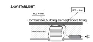
**Note:** LED driver can be placed under insulation, however, the driver's lifespan will be affected and warranty made void. Not suitable for use with loose-fill insulation.
