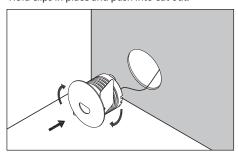
Note: Driver is too large to fit through ceiling cutout. Connect to fixed wiring before plasterboard is installed.
