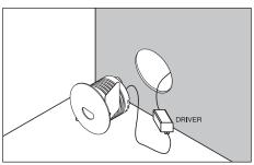
**Step 3** Hold clips in place and push into cut out.
