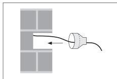
**Step 3** Ensure canister is level and flush with wall before rendering.
