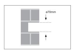
**Step 2**Run cable and push canister into wall.
